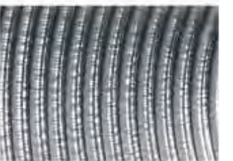
N12 R_a 50 \mu\text{m} – AARH / CLA 2000 R_z 185 \mu\text{m}
