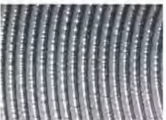
N11 R_a 25 \mu\text{m} – AARH / CLA 1000 R_z 102 \mu\text{m}
